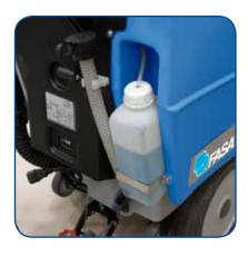
flow system. Easy access to recovery water tank with visual inspection. Extremely silent (62 dB) thanks to the particular housing of the vacuum motor and the use of soundproofing material.
